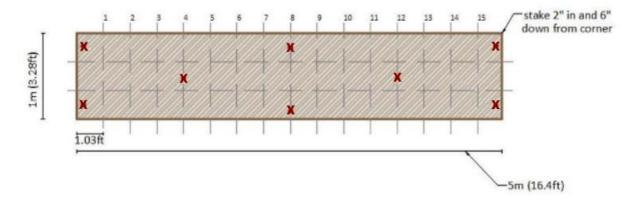
Staking requires overlapping ends and/or sides of two mats (2inches -4inches). Use 8 stakes; 2 on each end near the corners, 2 in the middle near the top and bottom, and 2 spaced evenly between the middle and the ends. If overlapped ends and/or sides, then move stakes closer to the edges (~2 inches from edge) to catch overlap of adjacent mats. Stakes should be inserted at an angle to pin coir fabric tightly to the ground until plants and leave about 4" of the stake protruding above the mat.
