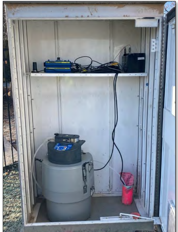
Photo 4 and 5: 11/8/23 - Photos are taken at south end of basin facing west. Photo shows newly installed monitoring station cabinet housing automated sampler and flow meter for stormwater sampling.
