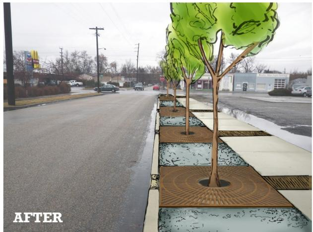
The structural component of the tree system profile allows installation of this compact GSI facility under structural roadway sections.
