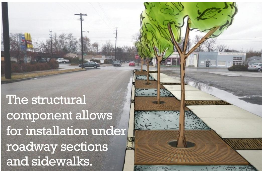
The structural component allows for installation under roadway sections and sidewalks.
